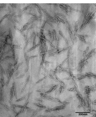
Transmission electron microscopy image CNCs.
