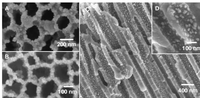
Figure 1. SEM images of silver nanoparticles on an alumina template. A) Silver nanoparticles on the top side of the template. B) Silver nanoparticles on the bottom side of the template. C) Cross section of alumina template showing silver nanoparticles on pore walls. D) Close-up of cross-section.
