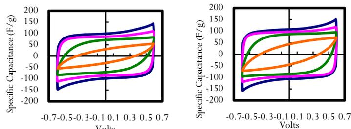
**Figure 1:** Cyclic voltammograms at scan rates of 1-500 mV/s for carbonization at (left) 700°C and (right) 900°C
