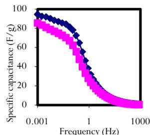
**Figure 2:** EIS frequency response for (top) 900°C and (bottom) 700°C
