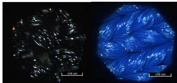
Figure 2: 50x magnification of, (A) Neoprene/Nylon, (B) Nylon/Spandex [3].
