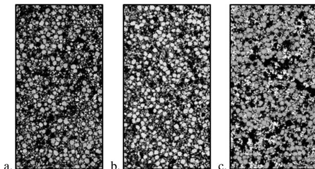
**Figure 1:** a) 60% density montage b) 70% density montage c) 80% density montage
