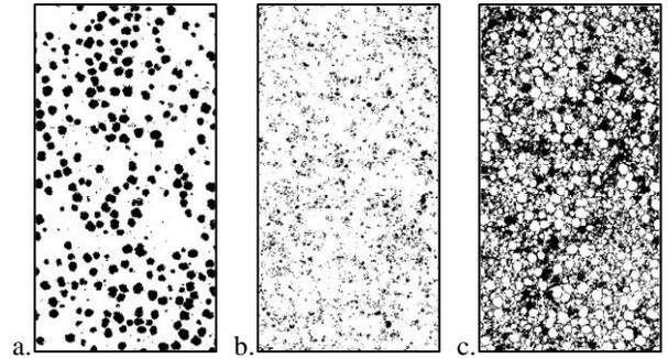
**Figure 2:** a) Segmented 60% with Ni in black b) Segmented 60% with Al in black c) Segmented 60% with voids in black
