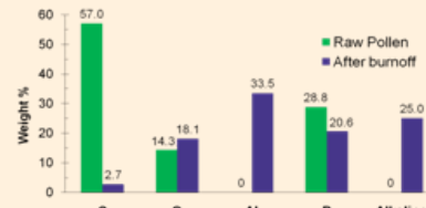
Figure 5: EDX Analysis of burnt coated pollen from Figure 3C indicating weight percent elemental composition
